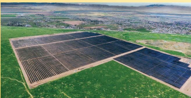
The pre-assembled drive system and easily assembled components combine to make for fast installs. The products offer high power density, with 99.5 percent panel density on rows. The trackers are very reliable, says the company, with rugged design for 30-year field life in harsh environmental climates.
