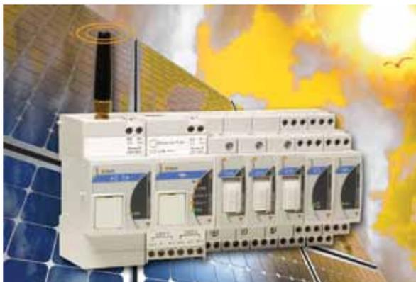
Full monitoring of solar plants is accomplished by the combination of the newly released VMU-C and VMU-W with the existing Eos-Array modules, the VMU-S, VMU-P, and VMU-O. The VMU-S string level monitoring module, the VMU-P environmental measurement module, and the VMU-O input/output modules split into independent modules. [www.GavazziOnline.com](http://www.GavazziOnline.com)
