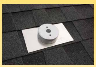
The Elevated Water Seal technology raises the water barrier 0.7 inches off the surface of the flashing and encases the EPDM sealing washer in a cast-aluminum block, isolating the EPDM sealing washer within its protective cavity. The flashing is 0.04 inches thick, which prevents distortion or bending of the flashing edges that can compromise waterproofing against wind-driven
