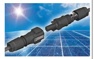
The one-piece DC connectors use spring technology for quick and easy assembly and termination without the use of crimp tools. The connectors can only be disconnected with the use of a screwdriver. This eliminates the possibility of accidental release, while meeting NEC requirements.
