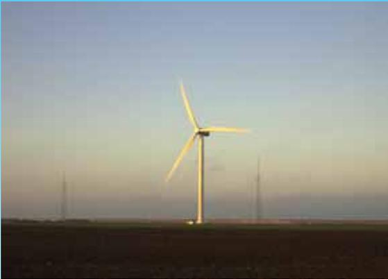
With a towerhead mass of roughly 350 tons, the SWT-6.0 is the lightest machine in its class, says the company. This unique combination of robustness and low weight significantly reduces infrastructure, installation, and service costs, and boosts lifetime energy output and profitability.
