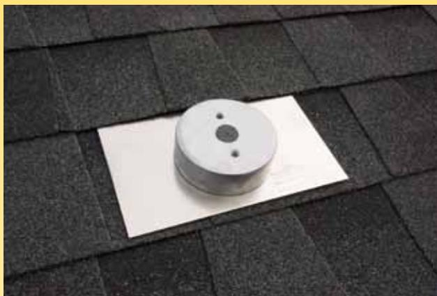
The Elevated Water Seal technology raises the water barrier 0.7 inches off the surface of the flashing and encases the EPDM sealing washer in a cast-aluminum block, isolating the EPDM sealing washer within its protective cavity. The flashing is 0.04 inches thick, which prevents distortion or bending of the flashing edges that can compromise waterproofing against wind-driven rain.
