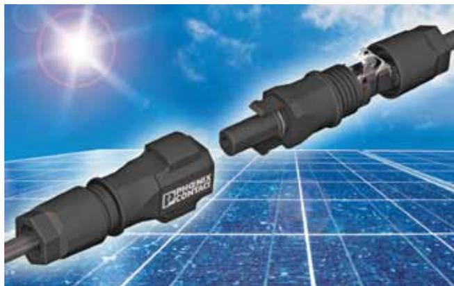
The one-piece DC connectors use spring technology for quick and easy assembly and termination without the use of crimp tools. The connectors can only be disconnected with the use of a screwdriver. This eliminates the possibility of accidental release, while meeting NEC requirements. [www.phoenixcontact.com](http://www.phoenixcontact.com)
